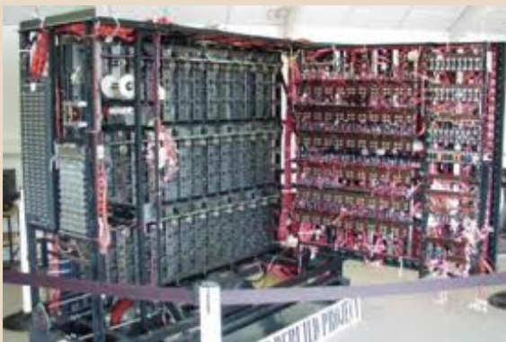
Bombe , designed by Alan Turing to decipher Enigma codes
